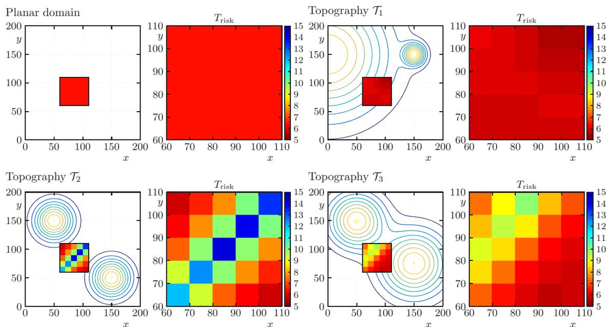
**Figure 13.** Scenarios 3.1 to 3.4: risk maps for the subdomain  $[60, 110] \times [60, 110]$  under the assumption of a flat domain (Scenario 3.1, top left) and domains with topography  $\mathcal{T}_1$ ,  $\mathcal{T}_2$ , and  $\mathcal{T}_3$  (Scenarios 3.2 to 3.4, top right, bottom left, and bottom right), visualizing for each patch of size  $10 \times 10$  the final time  $T_{\text{risk}}$ . A low value of  $T_{\text{risk}}$  implies a high risk.
