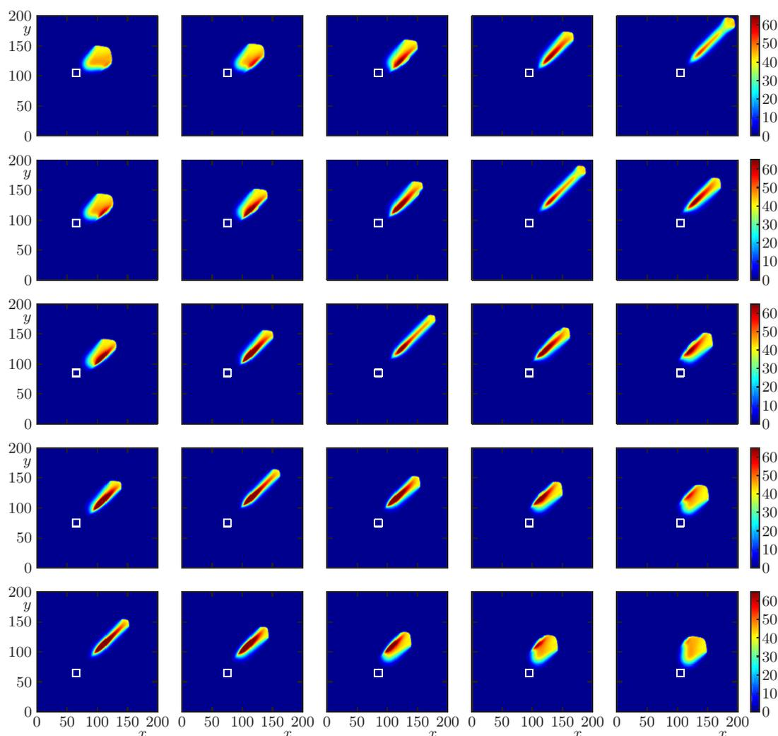
**Figure 9.** Scenario 3.3: simulation of temperature of a wildfire from  $5 \times 5 = 25$  initial fire foci, marked by small white squares, on a domain with topography  $\mathcal{T}_2$ .
