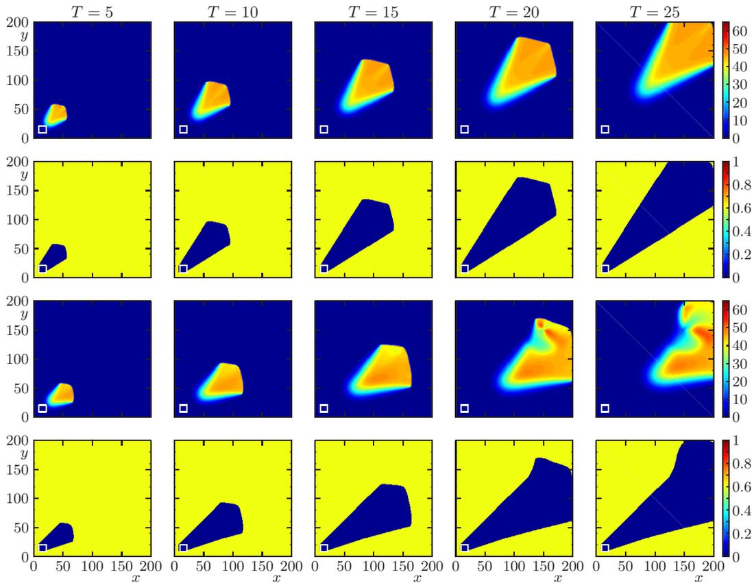
**Figure 4.** Scenarios 2.1 and 2.2: simulation of the propagation of a forest fire on a flat domain (first and second row) and on a domain with topography  $\mathcal{T}_1$  (third and fourth row), at indicated simulated times. Here and in Figure 5, the first and third row show temperature and the second and fourth row show fuel, and small white square indicates the location of the initial wildfire.
