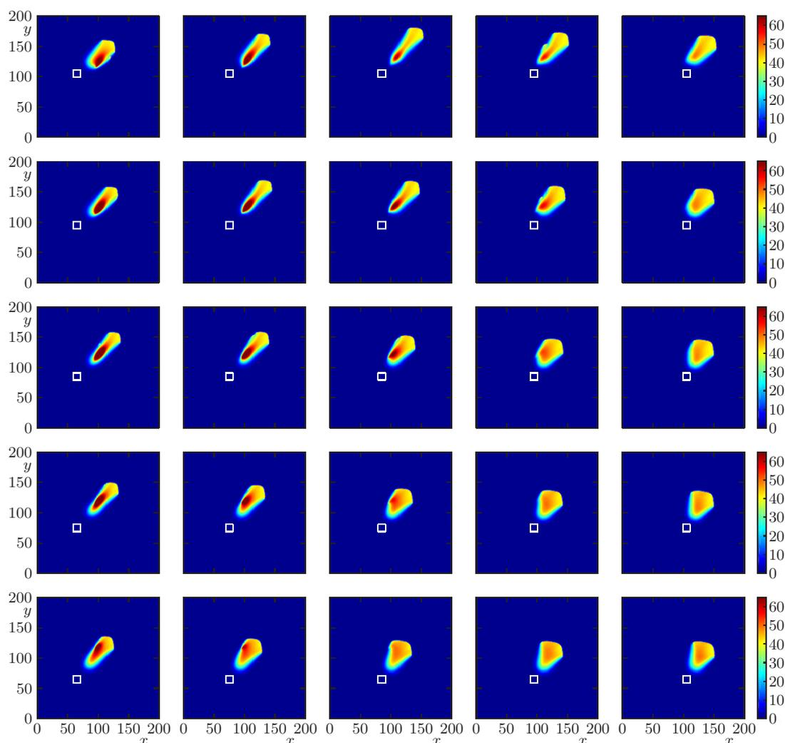
**Figure 11.** Scenario 3.4: simulation of temperature of a wildfire from  $5 \times 5 = 25$  initial fire foci, marked by small white squares, on a domain with topography  $\mathcal{T}_3$ .
