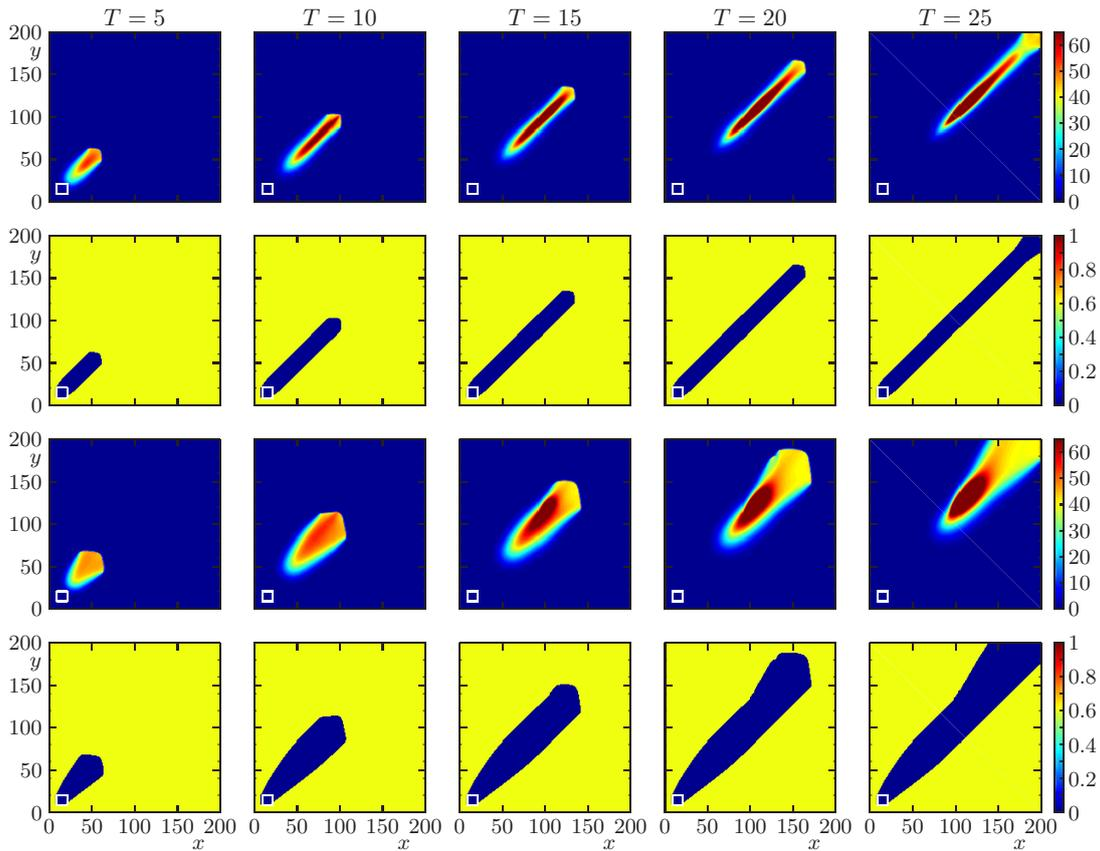
**Figure 5.** Scenarios 2.3 and 2.4: simulation of the propagation of a forest fire on domains with topographies  $\mathcal{T}_2$  (first and second row) and  $\mathcal{T}_3$  (third and fourth row).
