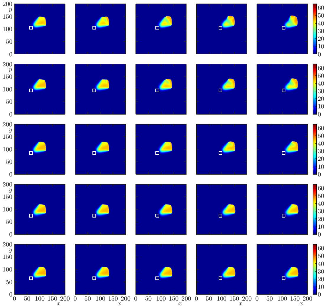
**Figure 7.** Scenario 3.2: simulation of temperature of a wildfire from  $5 \times 5 = 25$  initial fire foci, marked by small white squares, on a domain with topography  $\mathcal{T}_1$ . Here and in Figures 8 to 12, for each initial position the simulation is stopped, and the numerical solutions for  $u$  and  $v$  are portrayed, when 5% of the initially available fuel is burnt. The corresponding simulated time determines  $T_{\text{risk}}$  for each initial position.
