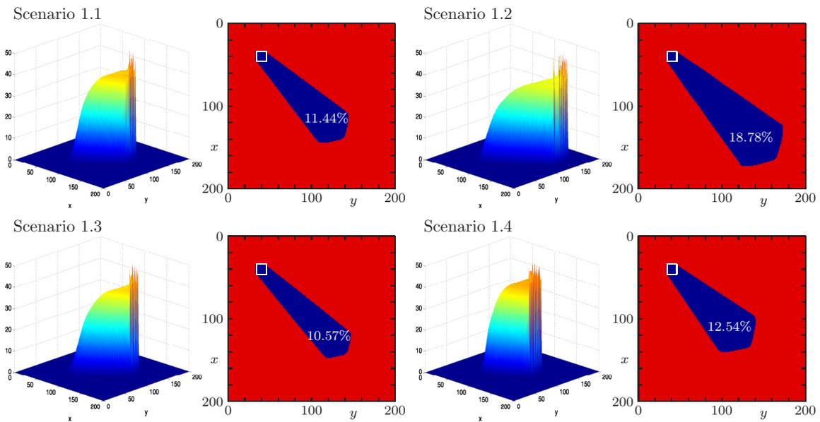
**Figure 2.** Scenarios 1.1 to 1.4: three-dimensional plots of simulated temperature and two-dimensional plots of simulated burnt fuel, at simulated time  $T = 12$ . The red and blue parts correspond to areas with  $v_0 = 0.9$  and  $v_0 = 0$ , respectively. The small white square indicates the location of the initial fire focus. The percentages represent the portion of burnt fuel of the total fuel initially available in  $\Omega$ .
