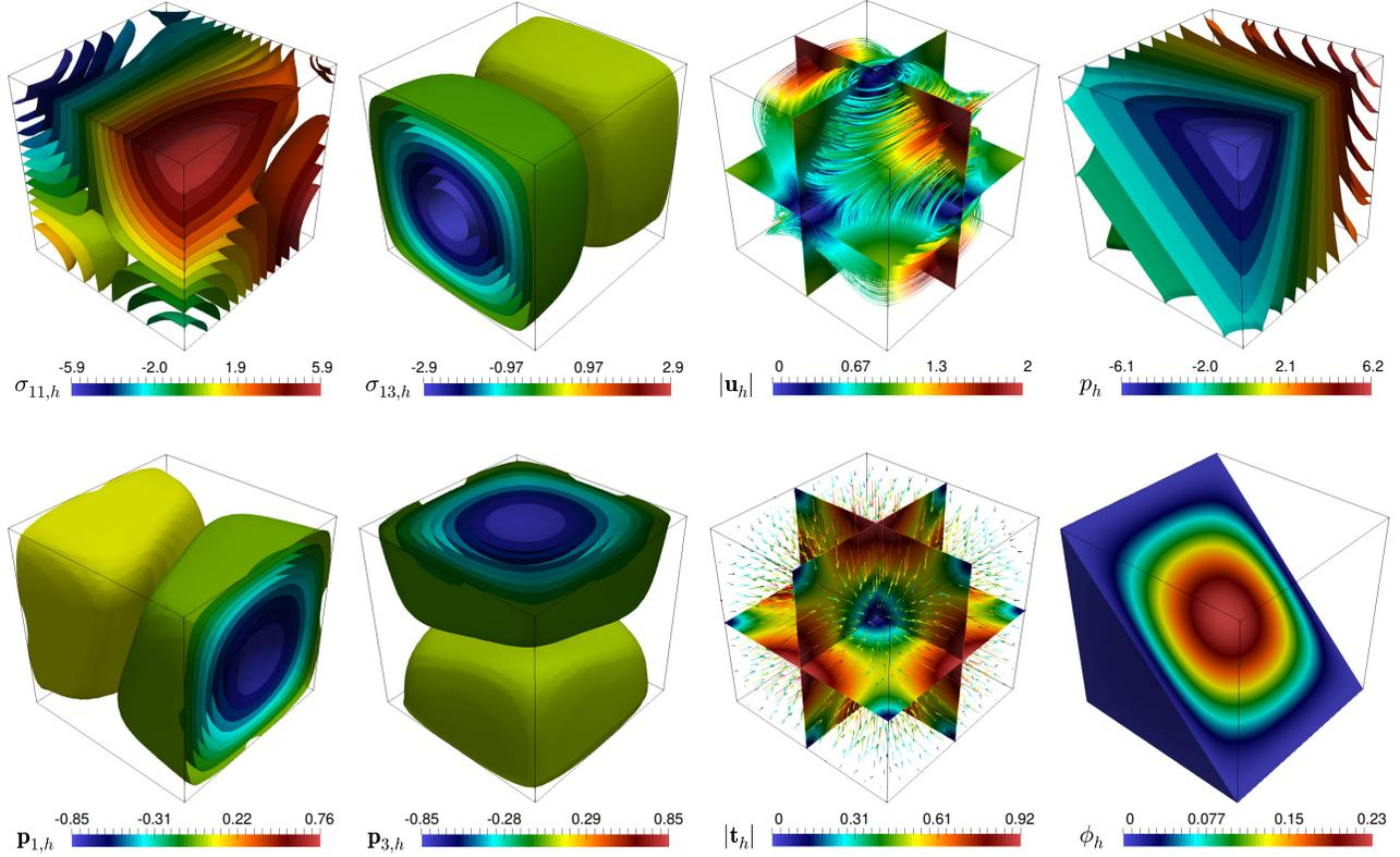
Figure 6.2: Example 2,  $\mathbb{RT}_0 - \mathbf{P}_0 - \mathbf{P}_0 - \mathbf{P}_0 - \mathbf{RT}_0$  approximation of Cauchy stress components, magnitude of the velocity, and pressure field (top plots); total flux components, magnitude of the concentration gradient and concentration field (bottom plots).
