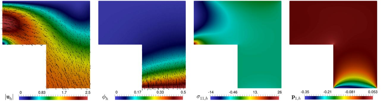
Figure 6.3: Example 3,  $\mathbb{RT}_0 - \mathbf{P}_0 - \mathbf{P}_0 - \mathbf{P}_0 - \mathbf{RT}_0$  approximation of the magnitude of the velocity, concentration field, first Cauchy stress component, and first total flux component.
