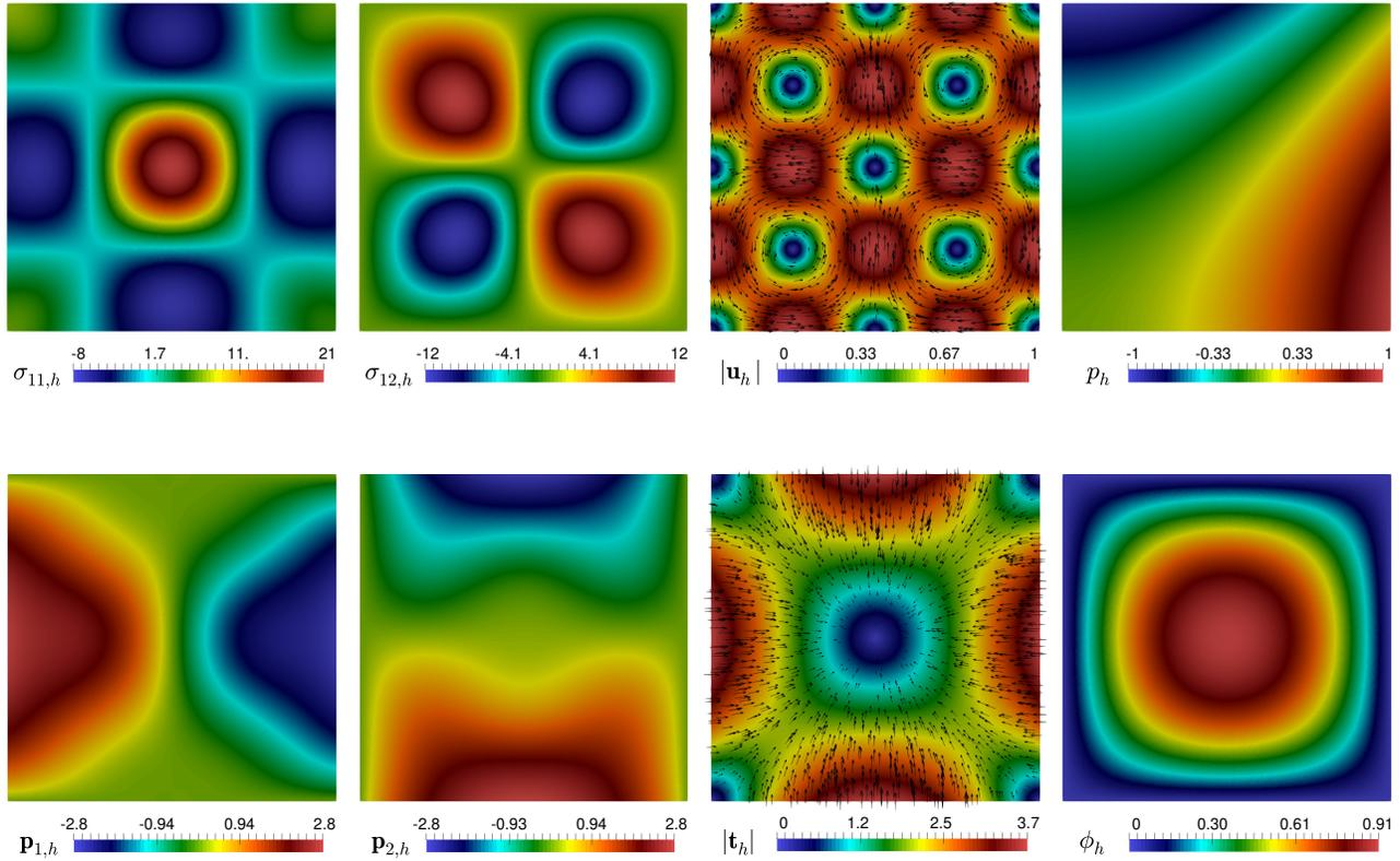
Figure 6.1: Example 1,  $\mathbb{RT}_1 - \mathbf{P}_1 - \mathbf{P}_1 - \mathbf{P}_1 - \mathbf{RT}_1$  approximation of Cauchy stress components, magnitude of the velocity, and pressure field (top plots); total flux components, magnitude of the concentration gradient and concentration field (bottom plots).
